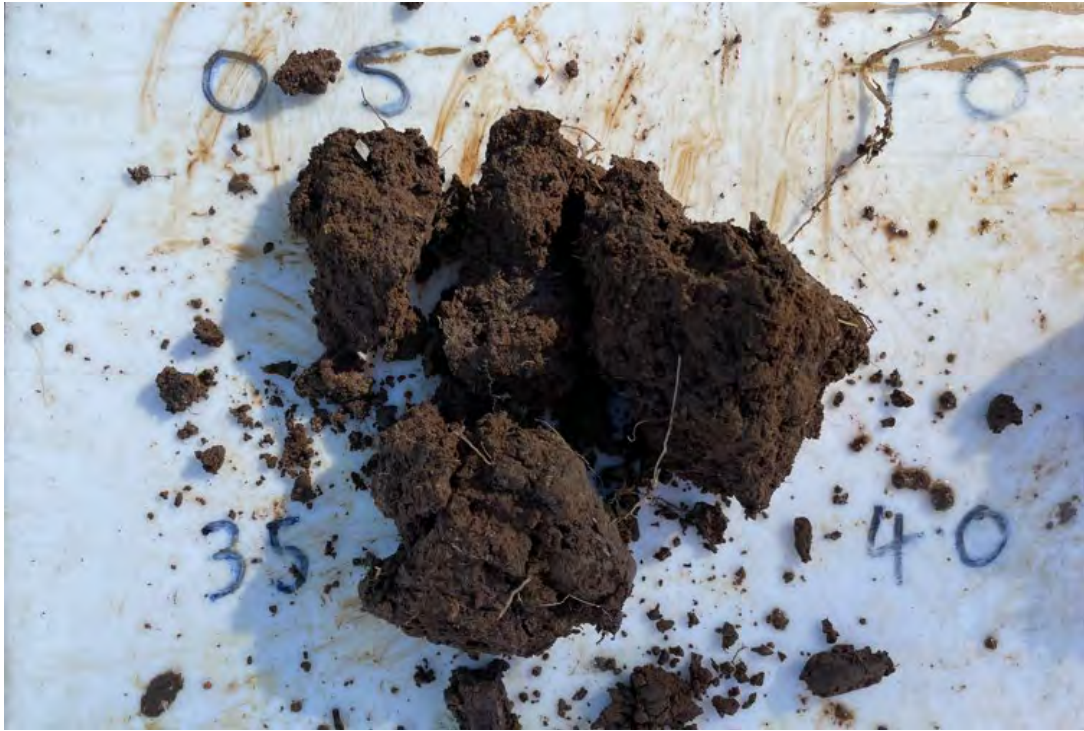
Photo 19 - Typical FILL (Silty CLAY) unit
